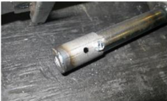
NG Air Collar Installed
